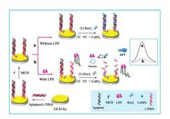
Electrochemical aptasensor based on DNAtemplated copper nanoparticles and RecJf exonuclease-assisted target recycling for lipopolysaccharide detection
