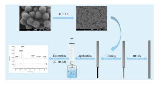
Facile fabrication of carbon nanotube hollow microspheres as a fiber coating for ultrasensitive solid-phase microextraction of phthalic acid esters in tea beverages
