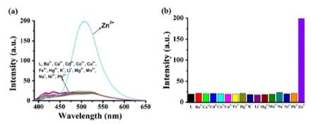
Fig. 4 (a) Emission spectra of probe 2 alone and with different metal ions. (b) Fluorescent intensity of 2 at 509 nm with different metal ions. Reproduced with permission from ref. 48. Copyright 2014 Springer.
