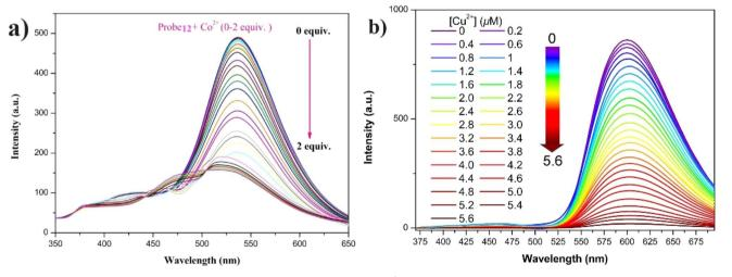
Fig. 18 (a) Emission spectra of probe 12 upon increasing concentrations of  $Co^{2+}$  ions in THF/H<sub>2</sub>O mixtures ( $f_w = 60\%$ , pH = 7.4,  $\lambda_{ex} = 330$  nm). (b) Emission spectra of probe 13 with increasing  $Cu^{2+}$  ions concentration in THF/H<sub>2</sub>O ( $f_w = 90\%$ , pH = 7.4,  $\lambda_{ex} = 350$  nm). Reproduced with permission from ref. 57. Copyright 2023 Springer.
