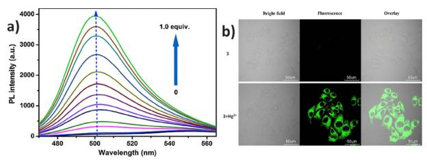
Fig. 6 (a) Emission spectra of probe 3 with increasing concentrations of  $Hg^{2+}$  ions in a DMSO/ $H_2O$  ( $f_w = 20\%$ ) mixture; (b) fluorescence images of HeLa cells treated with 3 and Hg<sup>2+</sup> ions. Reproduced with permission from ref. 49. Copyright 2015 Elsevier.
