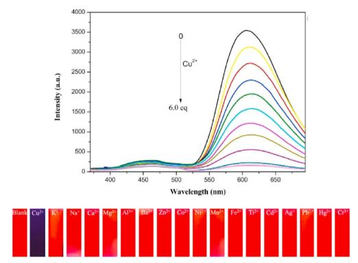
Fig. 14 Emission spectra of probe 9 upon increasing concentrations of  $Cu^{2+}$  ions in THF/H<sub>2</sub>O mixtures (v/v = 1:9, pH = 7.4,  $\lambda_{ex}$  = 350 nm) (top) and photographs of the silica gel testing strips for detecting various ions including under UV 365 nm illumination (bottom). Reproduced with permission from ref. 54. Copyright 2022 Elsevier.
