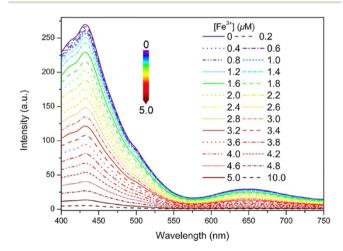
Fig. 22 Emission spectra of probe 16 (10  $\mu$ M) with various concentration of Fe<sup>3+</sup> ions in THF/water mixtures ( $f_{\rm w}=90\%$ , pH = 7.4,  $\lambda_{\rm ex}=380$  nm). Reproduced with permission from ref. 61. Copyright 2024 Elsevier.
