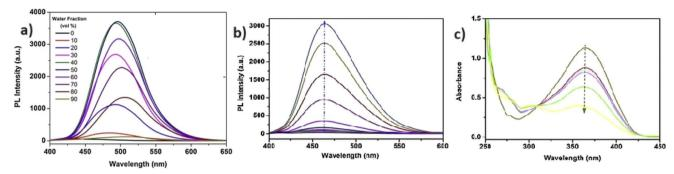
Fig. 2 (a) Emission spectra of probe 1 in THF $-H_2O$  mixtures; (b) change in the emission spectra of 1 upon increasing the concentrations of  $Hg^{2+}$  ions in THF; (c) absorption spectra of 1 upon increasing concentrations  $Hg^{2+}$  ions in THF. Reproduced with permission from ref. 47. Copyright 2014 Fisevier
