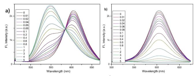
Fig. 10 (a) Fluorescence spectra of probe 6 with different concentrations of  $Zn^{2+}$  in THF/H<sub>2</sub>O (b) fluorescence spectra of probe 6 with different concentrations of  $Cu^{2+}$  ions in THF/H<sub>2</sub>O. Reproduced with permission from ref. 52. Copyright 2022 Elsevier.
