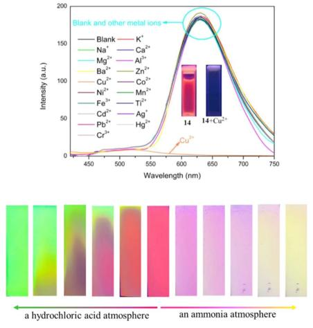
Fig. 20 Emission spectra changes of probe 14 in the presence of various metal cations (in THF/H<sub>2</sub>O system ( $f_w = 95\%$ , pH = 7.4,  $\lambda_{ex} = 400$  nm)) (top); fluorescence color responses of the TLC-based test strips loaded with probe 14 after exposure to HCl and NH<sub>3</sub> vapors for different times (bottom). Reproduced with permission from ref. 59. Copyright 2023 Elsevier.
