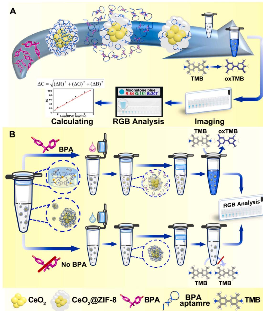
Fig. 3 (A) Diagrammatic description of the fabrication and the OXD-like properties of CeO<sub>2</sub>@ZIF-8/Apt nanoprobes. (B) The sensing mechanism of a one-pot portable testing substrate for bisphenol A determination. Reprinted with permission from ref. 80.
