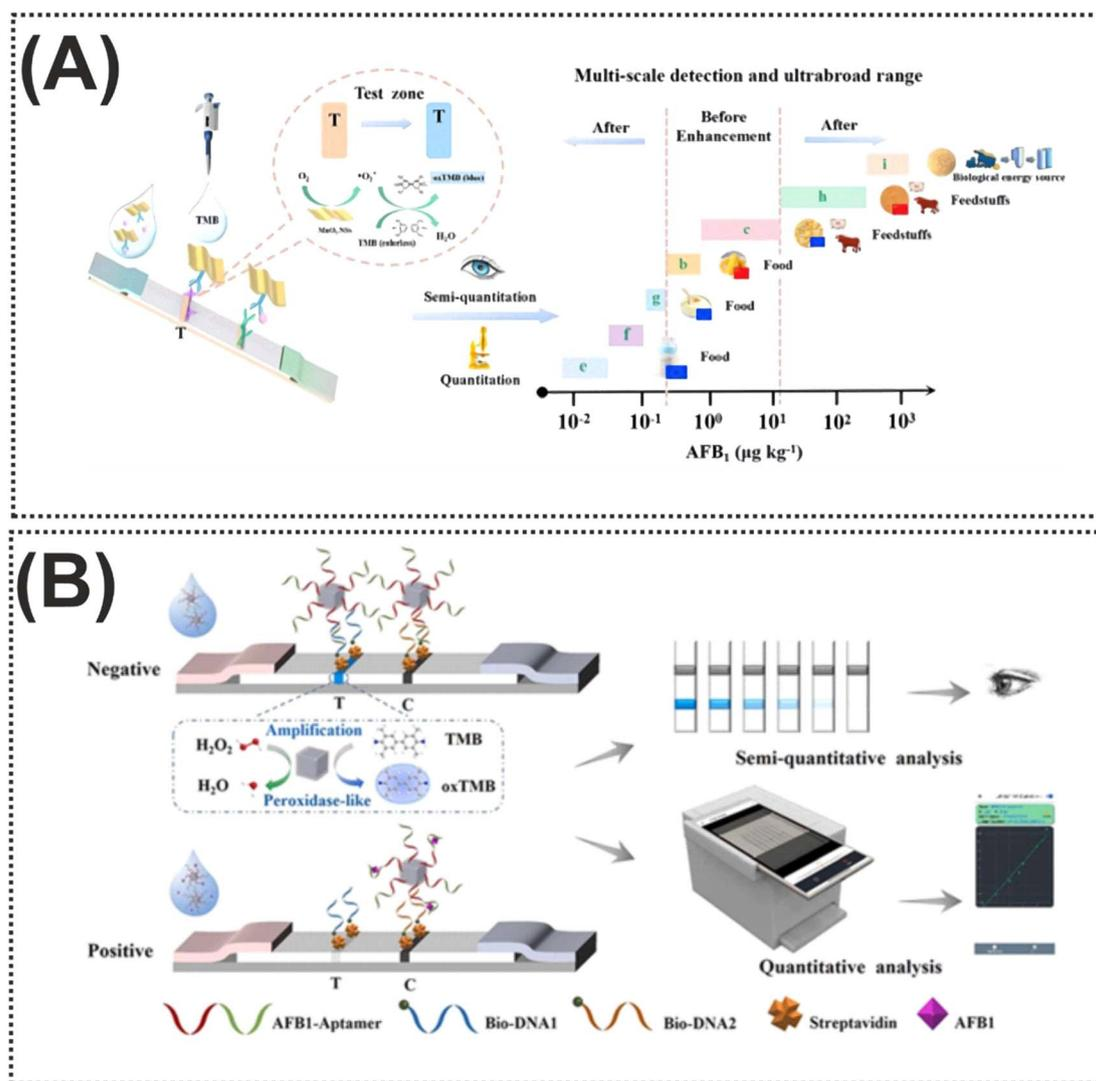
Fig. 6 (A) Schematic of the nanozyme-strip bioassay based on  $\text{MnO}_2$  NSs for AFB<sub>1</sub> detection. Reproduced with permission from ref. 99. Copyright Elsevier Science, 2022. (B) Illustration of the use of CuCo@PDA in the structure of LFA for AFB<sub>1</sub> quantification. Reproduced with permission from ref. 100. Copyright Elsevier Science, 2024.
