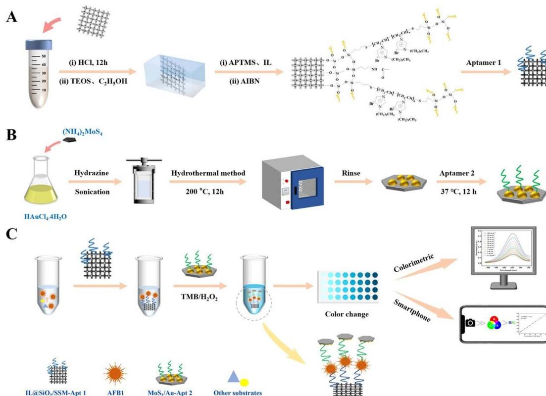
Fig. 4 (A–C) Representation of the colorimetric aptasensor based on MoS<sub>2</sub>/Au for AFB<sub>1</sub> determination. Reproduced with permission from ref. 94 Copyright Elsevier Science, 2024.
