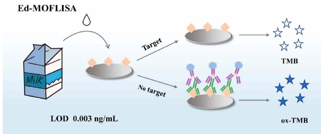
Fig. 7 Illustration of the application of NanoMOFs for colorimetric detection of AFB<sub>1</sub>. Reproduced with permission from ref. 106. Copyright Elsevier Science, 2022.
