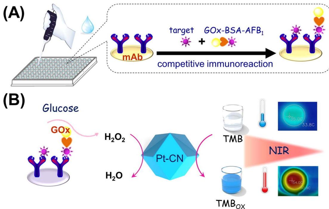
Fig. 5 (A) Competitive immunosensor exploiting the GOx-labeled AFB<sub>1</sub>-BSA conjugate as the tag. (B) Illustration of colorimetric and photothermal measurement based on H<sub>2</sub>O<sub>2</sub>-responsive peroxidase-like activity of Pt-CN. Reproduced with permission from ref. 95. Copyright Elsevier Science, 2019.
