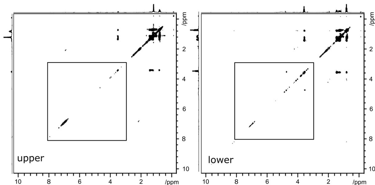
Fig. 2 2D  $^1\text{H}$  TOCSY spectra of three-component separated sample B. Left-hand spectrum depicts the upper layer and right-hand spectrum depicts the lower layer. Spectral regions indicated by boxes are reproduced, enlarged, in Fig. 3.
