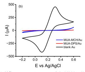
Fig. 1 (a) Chronoamperometry responses of mixed thiol deposition on Au electrodes held at +0.5 V vs. Ag/AgCl in a solution containing MUA-MCH and MUA-DPS; (b) CVs of 1 mM [Fe(CN)<sub>6</sub>]<sup>3-/4-</sup> in 0.1 M PBS, pH 7.4 using a bare Au and electrodeposited MUA-MCH and MUA-DPS SAMs modified Au electrodes.
