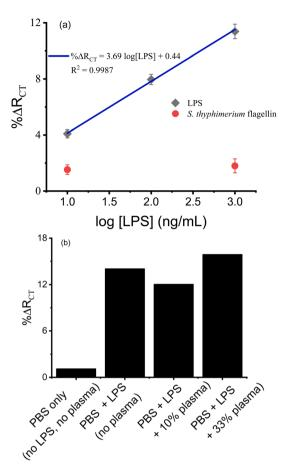
Fig. 4 (a) Dose–response curve of TLR4/MUA-DPS/Au towards LPS. Response of the sensor towards control samples (10 and 1000 ng mL<sup>-1</sup> flagellin from *Salmonella typhimurium*) is shown with red circles; (b) the response of the TLR4 sensor (TLR4/MUA-DPS/Au) for 1000 ng mL<sup>-1</sup> LPS spiked pooled human blood plasma samples. The data points and error bars represent the mean and standard deviation of three independent sensors fabricated and processed in parallel.
