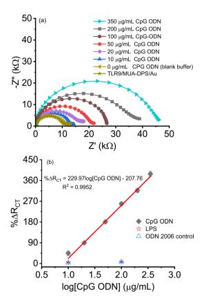
Fig. 6 (a) Nyquist plot of the TLR9/MUA-DPS/Au sensor after 30 minute incubation with various concentrations of CpG ODN. The amount of CpG ODN ( $\mu$ g mL $^{-1}$ ) used to generate each EIS data point is indicated in the plot; (b) calibration plot of % $\Delta R_{CT}$  of the TLR9 biosensor as a function of logarithm of CpG ODN concentration. Data points and error bars represent the mean and standard deviation of three independent sensors fabricated and processed in parallel.
