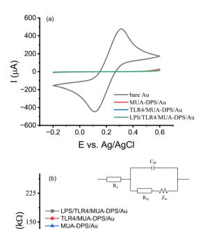
Fig. 2 Cyclic voltammograms (a) and Nyquist plots (b) of the Au electrode following the steps in TLR sensor fabrication using 1 mM [Fe(CN)<sub>6</sub>]<sup>3-/4-</sup> prepared in PBS buffer (pH = 7.4). Inset in (b) also shows the Randles equivalent circuit used for all fits.  $R_{\rm s}$  is the solution resistance;  $C_{\rm dl}$  is the electrode double layer capacitance;  $Z_{\rm w}$  is the Warburg impedance and  $R_{\rm CT}$  is the charge transfer resistance at the electrode interface.
