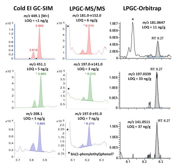
Fig. 5 Comparison in the analysis of 100 ng  $g^{-1}$  (75 pg injected)  $\lambda$ -cyhalothrin in the barley extract using different fast GC-MS techniques. In MS/ MS, the peak with  $t_R = 6.06$  min is the same chemical as shown in Fig. 2 and S2 (ESI‡), but the missing m/z 197 fragment ion in HRMS demonstrates that it has a different elemental composition than  $\lambda$ -cyhalothrin.
