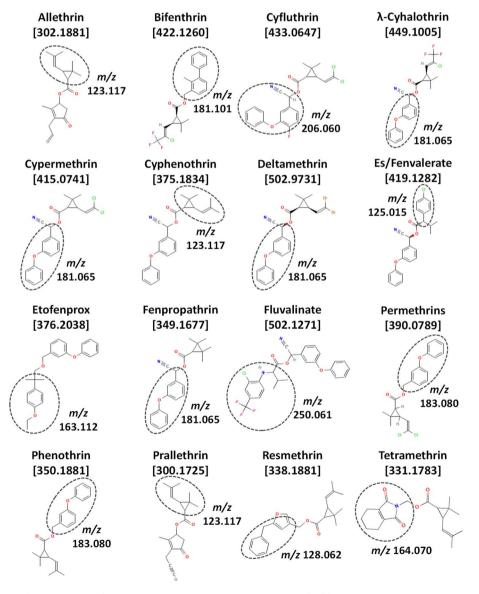
Fig. 1 Chemical structures (from PubChem), exact mass monoisotopic molecular ions (m/z), and standard EI-MS base peak fragment ions of the 16 pyrethroids in this study, including prallethrin.
