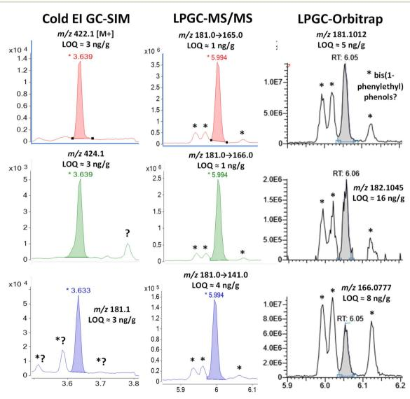
Fig. 4 Comparison in the analysis of  $100 \text{ ng g}^{-1}$  (75 pg injected) bifenthrin in the barley extract using different fast GC-MS techniques. The peaks marked with \* were identified as 2,4-bis(1-phenylethyl)phenol by LPGC-orbitrap using the NIST library (see Fig. S3‡), and the 3 peaks presumably consist of the 2,4-, 2,5-, and 3,5-structural isomers originating from nitrile gloves.
