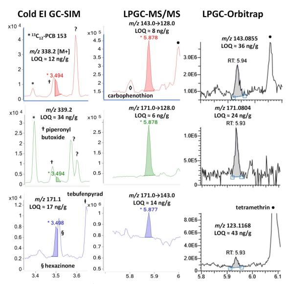
Fig. 11 Comparison in the analysis of 100 ng  $g^{-1}$  (75 ng injected) resmethrin in the barley extract using different fast GC-MS techniques. Other pesticides added to the mixture posed problems with fast-GC Cold EI-SIM, but not LPGC MS/MS or HRMS (orbitrap),
