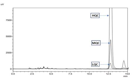
Fig. 4 Overlay of chromatograms for LQC, MQC, and HQC samples of AKBA.
