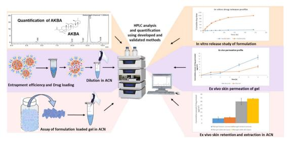
Fig. 1 Diagrammatic representation of the application of the developed RP-HPLC chromatographic method.
