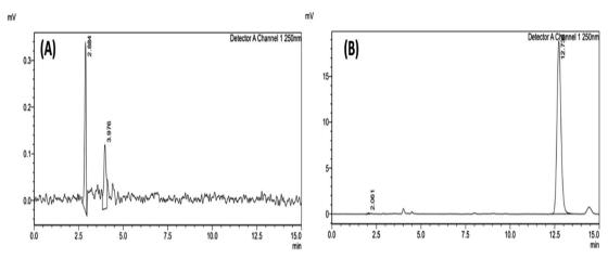
Fig. 2 (A) Chromatogram of blank ACN and (B) chromatogram of 10 000 ng mL<sup>-1</sup> AKBA sample
