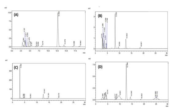
RP-HPLC chromatogram of (A) acid hydrolysis, (B) base hydrolysis, (C) oxidative hydrolysis, and (D) thermolytic hydrolysis.
