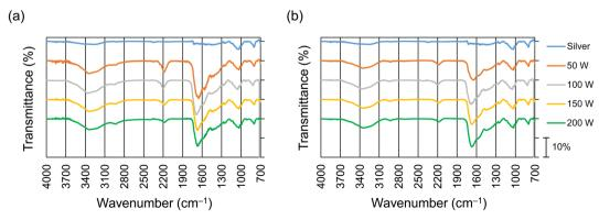
Fig. 4 Influence of RF power on FTIR spectra (a) prior to and (b) after washing.
