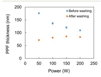
Fig. 3 Influence of RF power on PPF thickness. The error bars indicate the standard deviation of five measurements.
