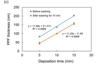
Fig. 2 Influence of washing of PPFs on (a) thickness, (b) FTIR spectra, and (c) the relationship between deposition time and PPF thickness. PPFs were deposited on silicon chips (a) and silver-coated glass slides (b). The error bars in (a) and (c) indicate the standard deviation of five measurements.
