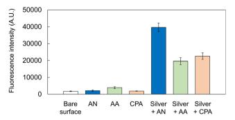
Fig. 6 Influence of monomers (acetonitrile (AN), allylamine (AA), and cyclopropylamine (CPA)) on fluorescence enhancement using immobilized Oligo-Cy5-SH. The error bars indicate the standard deviation of four measurements.
