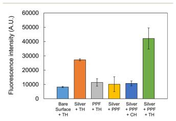
Fig. 7 Aptamer sandwich assay for thrombin (TH) on multilayered glass slide. Chymotrypsin (CH) was used as a control. The error bars indicate the standard deviation of four measurements.
