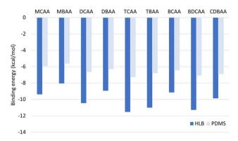
Fig. 3 Computationally determined binding energies of the most stable protonated HAA conformers interfaced with a monomer of each sorbent (HLB and PDMS).
