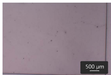
Fig. 5 Light micrograph of the PDMS thin film.
