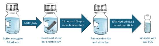
Fig. 1 Flow chart of the experimental procedure used to compare thin film extraction efficiency.
