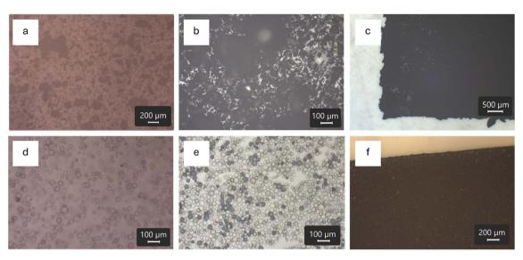
Fig. 6 Light micrographs of thin films prepared with sorbents. (a)—(c) Carboxen® impregnated PDMS films. (a) Lower mass of sorbent added. (b) Greater mass of sorbent added. (c) Sorbent on the film surface. (d)—(f) HLB impregnated PDMS films. (d) Lower mass of sorbent added. (e) Greater mass of sorbent added. (f) Sorbent on the film surface.
