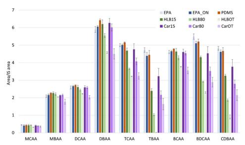
Fig. 7 Averages of triplicate area ratios of spiked deionized water, extracted with different thin film types, followed by processing and analysis with EPA Method 552.3. Outliers were determined with the *z*-score and error bars represent the standard deviation.
