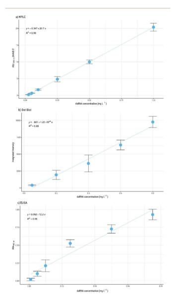
Fig. 2 dsRNA calibration curves and corresponding linear regression obtained for the analytical method used: HPLC (a), dot blot (b) and ELISA (c). Three independent linear regression analyses were performed, and 3 independent samples were analysed.
