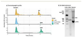
Fig. 1 Analysis of dsRNA by RP-HPLC and corresponding gel electrophoresis of the samples. (a) Chromatographic profile of total mRNA (yellow) and dsRNA before (blue) and after purification (green) obtained by the developed RP-HPLC method. (b) Agarose gel electrophoresis of the total mRNA (initial) and after digestion with RNase T1 (digested).
