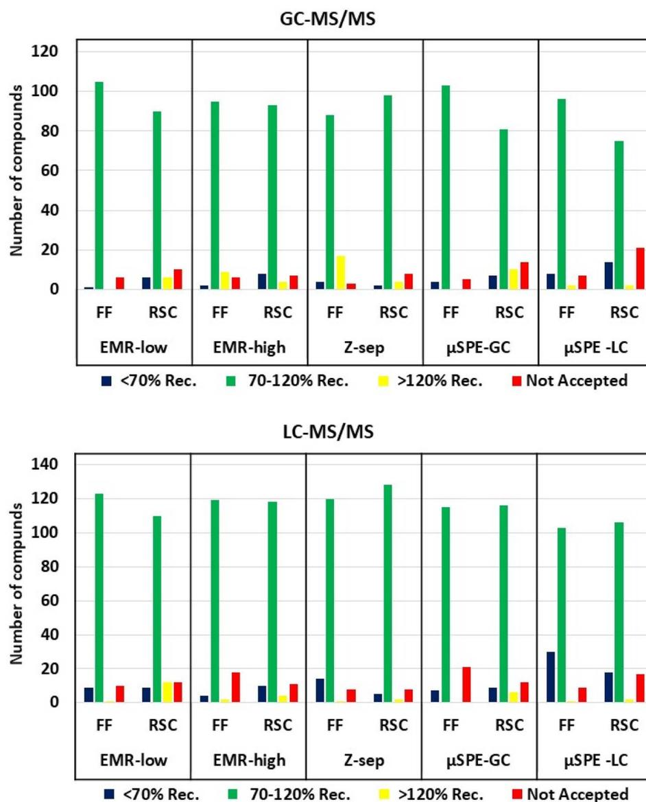
Fig. 4 Number of compounds within different ranges of recoveries at a spiking level of 0.01 mg kg<sup>-1</sup> ( $n = 5$ ) in both matrices, FF and RSC. The number of compounds analyzed is 123 by GC and 143 by LC. Not accepted are all the compounds that either could not be detected or whose RSD was higher than 20%.
