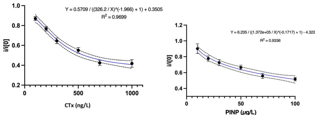
Fig. 10 Calibration curve of CTx and PINP immunosensors inside the microsystem housing. 10 mM PBS pH 7.4 containing 0.1 M KCl and 0.5 mM  $[\text{Fe}(\text{CN})_6]^{3-/4-}$  (1 : 1) was used as the electrolyte solution for the electrochemical readings. Calibration curve fitting was done using the 4 PL method.
