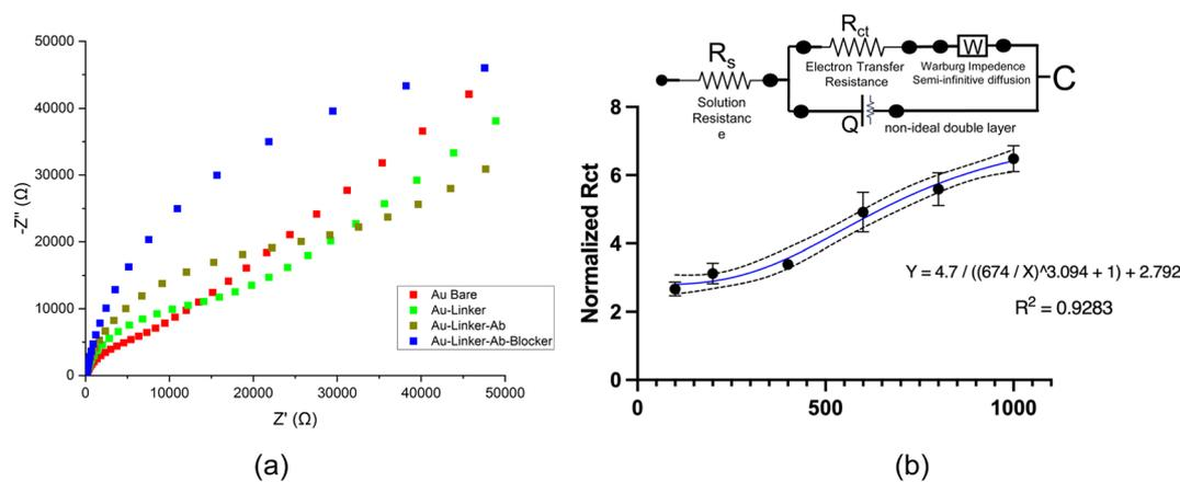
Fig. 6 Nyquist plots showing successful the layer-by-layer deposition on the sensing layer measurements performed at  $0.2 \text{ V}$  in  $\text{K}_4[\text{Fe}(\text{CN})_6]/\text{K}_3[\text{Fe}(\text{CN})_6]$  over a frequency range of  $0.1 \text{ Hz}$  and  $0.1 \text{ MHz}$ . Inset: Randles equivalent circuit ( $R[Q(RW)]$ ) representing the sensing layer of the immunosensor. Calibration curve fitting is done using the 4 PL method.
