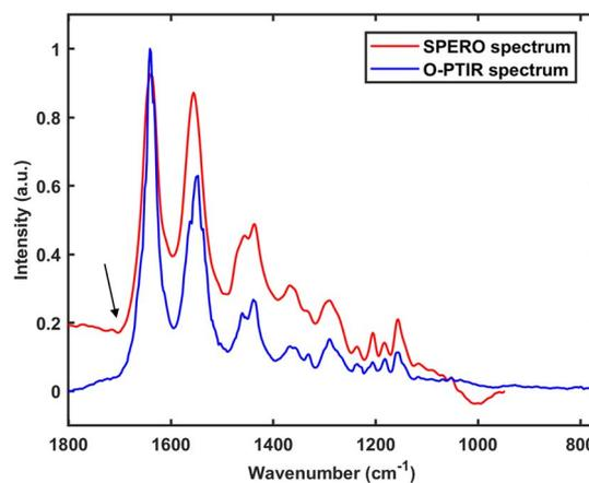
Fig. 6 A spectrum of a 10  $\mu\text{m}$  nylon particle obtained using the SPERO microscope in transmission mode and an O-PTIR spectrum of another 10  $\mu\text{m}$  nylon particle. The spectral range of the SPERO spectrum is 1900–948  $\text{cm}^{-1}$ . The spectral range of the O-PTIR spectrum is 1801–769  $\text{cm}^{-1}$ . The black arrow indicates where a first derivative-like line shape could be seen in the SPERO spectrum.
