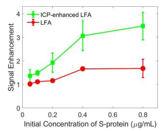
Fig. 7 A calibration curve comparing the signal enhancement of the region containing the test line at t=40 min for five initial concentrations of S-protein for an LFA with enrichment (blue) and an LFA without enrichment (red). For the LFA with enrichment, the voltage was ramped from 1.0 to 80.0 V at a rate of 1.0 V per 10 s for a total time of 30 min. The error bars represent 1 standard deviation of the signal enhancement from 3 replicates.
