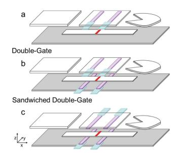
Scheme 3 Schematic of the three configurations of Nafion-coated electrodes - (a) double-gate, (b) sandwiched double-gate, and (c) flipped sandwich double-gate configurations.
