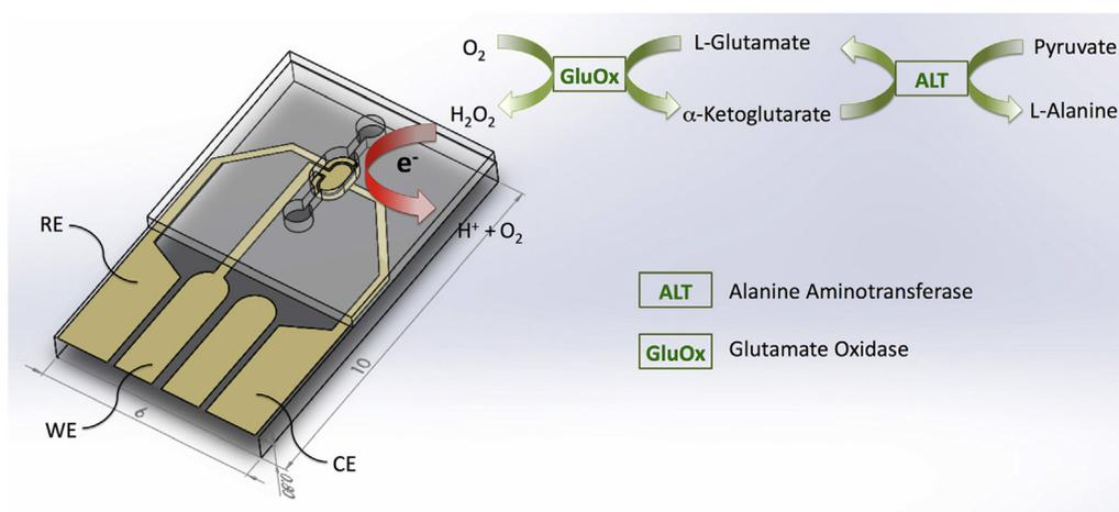
Fig. 3 Illustration of ALT detection on the Pt thin-film electrode.<sup>27</sup>
