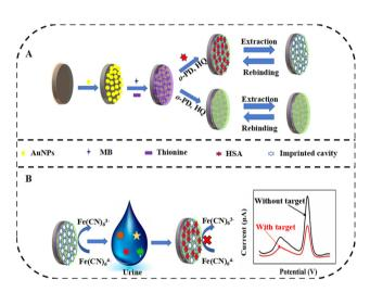
Fig. 2 Schematic of (A) MIP-based sensor construction and (B) electrochemical detection of HSA.<sup>13</sup>
