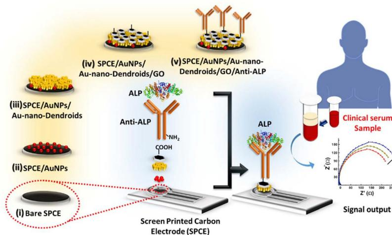
Fig. 1 Illustration of ALP detection on the composite electrode.<sup>33</sup>
