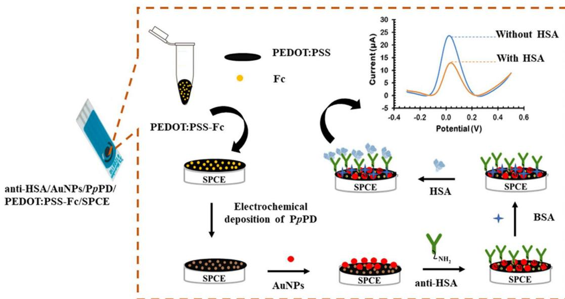
Fig. 4 Illustration of HSA detection.<sup>39</sup>
