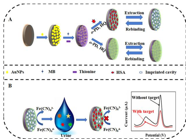
Fig. 2 Schematic of (A) MIP-based sensor construction and (B) electrochemical detection of HSA.<sup>13</sup>
