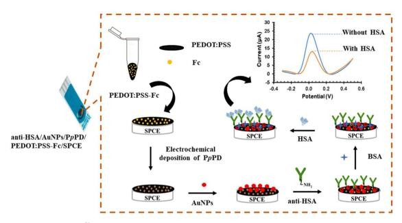
Fig. 4 Illustration of HSA detection.<sup>39</sup>
