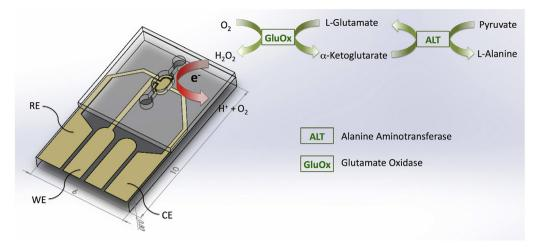
Fig. 3 Illustration of ALT detection on the Pt thin-film electrode.<sup>27</sup>
