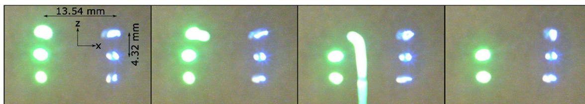
Fig. 4 Montage of images showing falling of a droplet while merging two lines of levitated droplets where time resolution is 454 ms.
