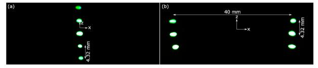
Fig. 2 Levitated 2 µl droplets of 10 ppm fluorescein in PBS at (a) a single focus at [0, 0, 0] and (b) two foci at [-20, 0, 0] and [20, 0, 0] (both: mm).
