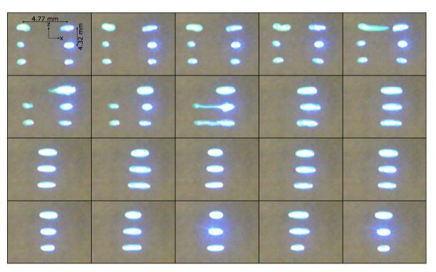
Fig. 5 Montage of images showing successful merging of two lines of levitated droplets where time resolution is 227 ms (images should be read from top left to right and then from top to bottom row and droplets were moved towards each other at 0.5 mm s<sup>-1</sup>).
