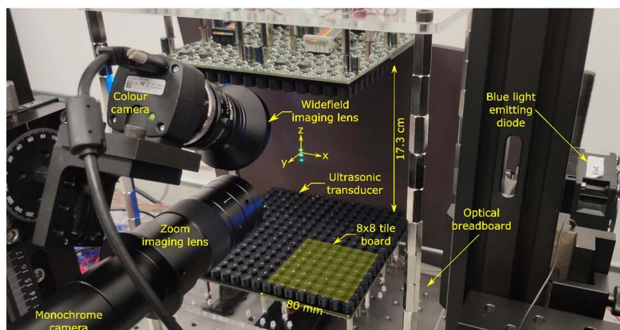
Fig. 1 Schematic of our acoustic levitator with integrated optical detection system.
