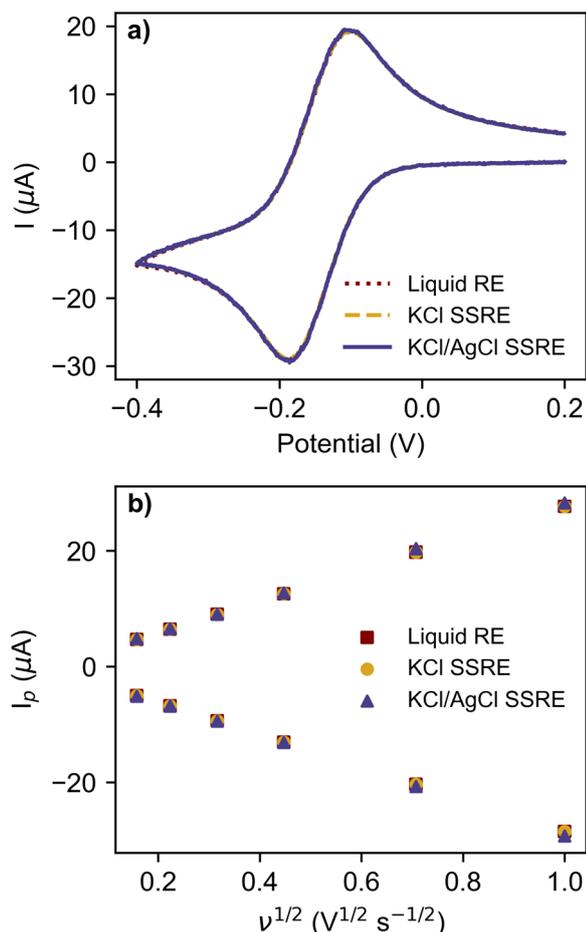
**Fig. 4** (a) cyclic voltammograms using a  $1 \text{ V s}^{-1}$  scan rate with  $5 \text{ mM}$   $[\text{Ru}(\text{NH}_3)_6]\text{Cl}_3$  and  $0.2 \text{ M}$  KCl supporting electrolyte using a  $1 \text{ mm}$  diameter GC electrode with a liquid RE, KCl SSRE, and KCl/AgCl SSRE. (b) Peak currents ( $I_p$ ) vs. square root of scan rate ( $\nu$ ) for voltammograms measured using various reference electrodes.
