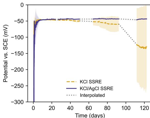
**Fig. 5** long term potential monitoring of KCl SSRE and KCl/AgCl SSREs in  $1 \text{ g L}^{-1}$   $\text{Na}_2\text{S}$  solution in pH 9 buffer. Mean potentials ( $n = 5$ ) are reported with the coloured shading indicating the 95% confidence interval. Interpolated sections indicate periods where the conventional SCE reference suffered sulphide poisoning.
