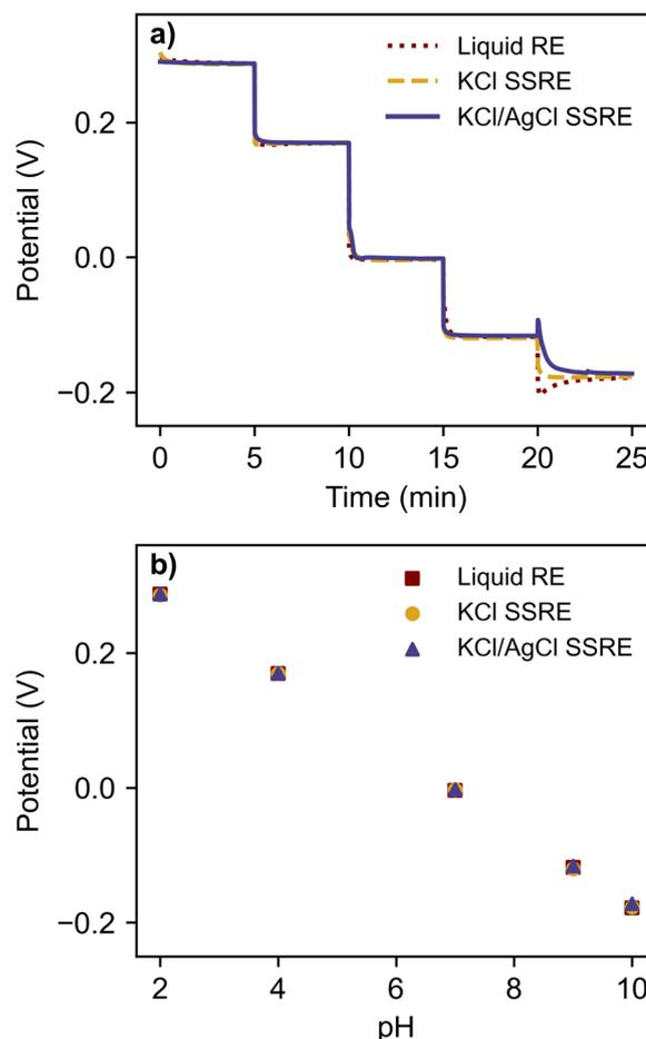
Fig. 3 (a) open circuit potentiometry with glass pH electrode in a series of pH buffers using a liquid RE, KCl SSRE, and KCl/AgCl SSRE, and (b) the resulting calibration curve.
