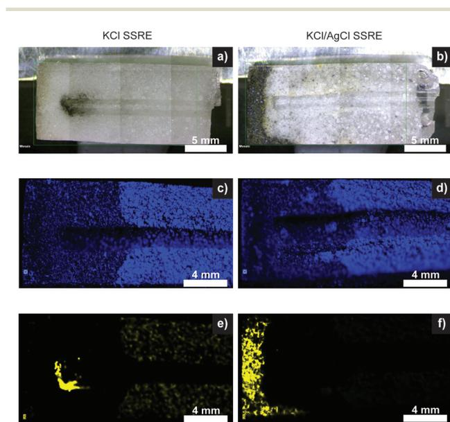
**Fig. 6** KCl SSRE (left column) and KCl/AgCl SSRE (right column) cross section images (a and b) and  $\mu$ XRF mapping of chlorine (c and d) and sulphur (e and f) after long term potential monitoring in 1 g L<sup>-1</sup> Na<sub>2</sub>S solution.
