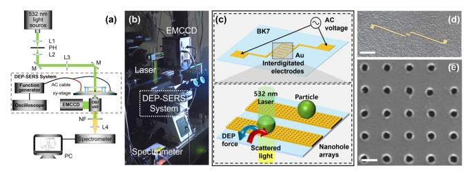
Fig. 1 (a) Schematic representation of the optical set-up (M: mirrors, L1-L4: lenses, PH: pinhole, OBJ: objective lens, NF: notch filter, and light source  $\lambda$  = 532 nm). (b) Photograph of the constructed DEP-SERS system. (c) Schematic representations of a DEP-SERS chip. (d) Photograph of a DEP-SERS chip (scale bar: 4 mm). (e) SEM image of fabricated nanohole arrays (diameter: 250 nm and period: 700 nm, scale bar: 500 nm).
