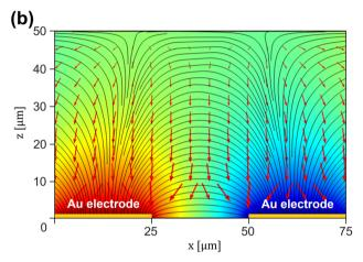
Fig. 3 (a) Simulation of the electric field generated by IDEs composed of gold, with each electrode having a width of 25 µm and separated by a 25 µm gap. (b) Cross-sectional view along the x-axis of the electric field and DEP force vectors. The arrows indicate the direction of the positive DEP force vectors acting on a cell with a diameter of 10 µm.
