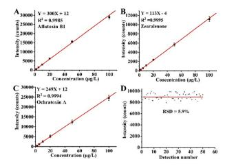
Fig. 4 (A–C) Calibration curves for aflatoxin B1, zearalenone and ochratoxin A, with the intensity of the  $[M+H]^+$  peak plotted as a function of injected concentration. (D) Aflatoxin B1 was tested repeatedly, 50 times
