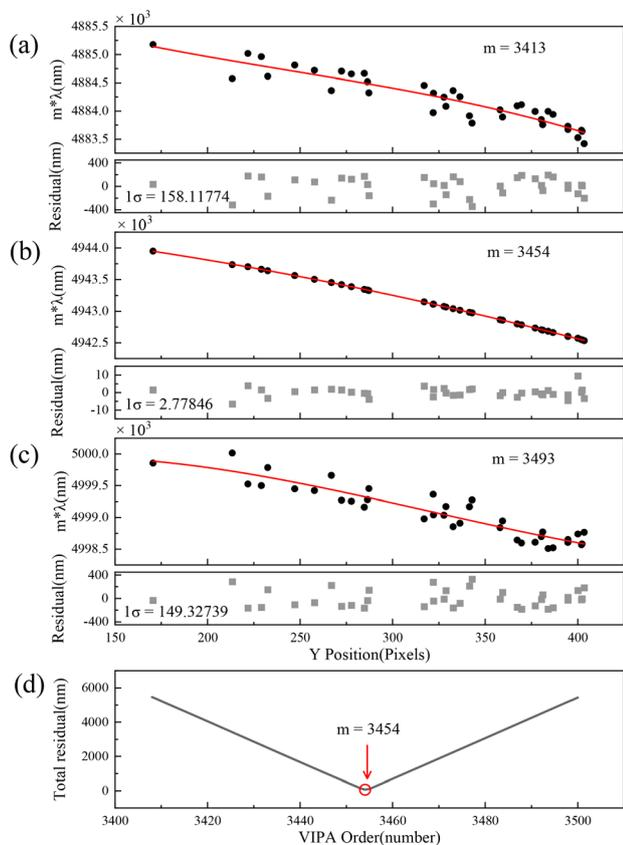
**Fig. 5** Schematic diagram of the inversion of optimized model parameters. The second-order polynomial fitting results under the conditions of (a)  $m = 3413$ , (b)  $m = 3454$ , and (c)  $m = 3493$ . (d) The sum of the fitting residuals at different  $m$  values.
