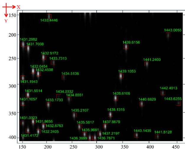
Fig. 7 Zoomed-in CO<sub>2</sub> absorption image. Absorption spots within a VIPA FSR are labelled with their wavelength.
