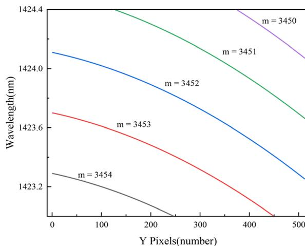
**Fig. 6** Theoretical spectrum calculated by fitting parameters with different  $m$  values. Different lines (different  $m$  values) represent different fringes on the detector plane. The  $X$  coordinate of the pixel can be obtained by the fringe recognition algorithm. The  $Y$  coordinate of the pixel and its wavelength can be obtained from the curve, and thus the wavelength corresponding to each central pixel on the fringe can be obtained.
