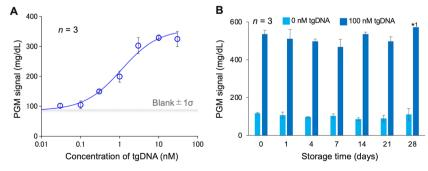
Fig. 5 (A) Relationship between tgDNA concentration and PGM signal after 60 min of CRISPR reaction time and another 60 min of invertase reaction time. (B) Storage stability of the fully integrated device at -20 °C; error bars represent the mean values  $\pm 1\sigma$  (n = 3); the result without an error bar includes signals above the detection range of the PGM (521, 596 and >600 mg  $dL^{-1}$ ).
