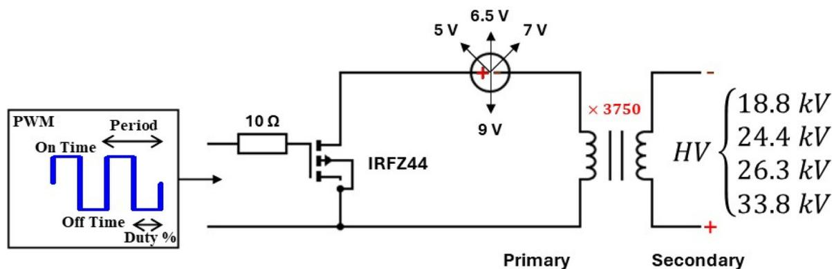
Fig. 2 Schematic diagram of the power supply of HA-DBDI.
