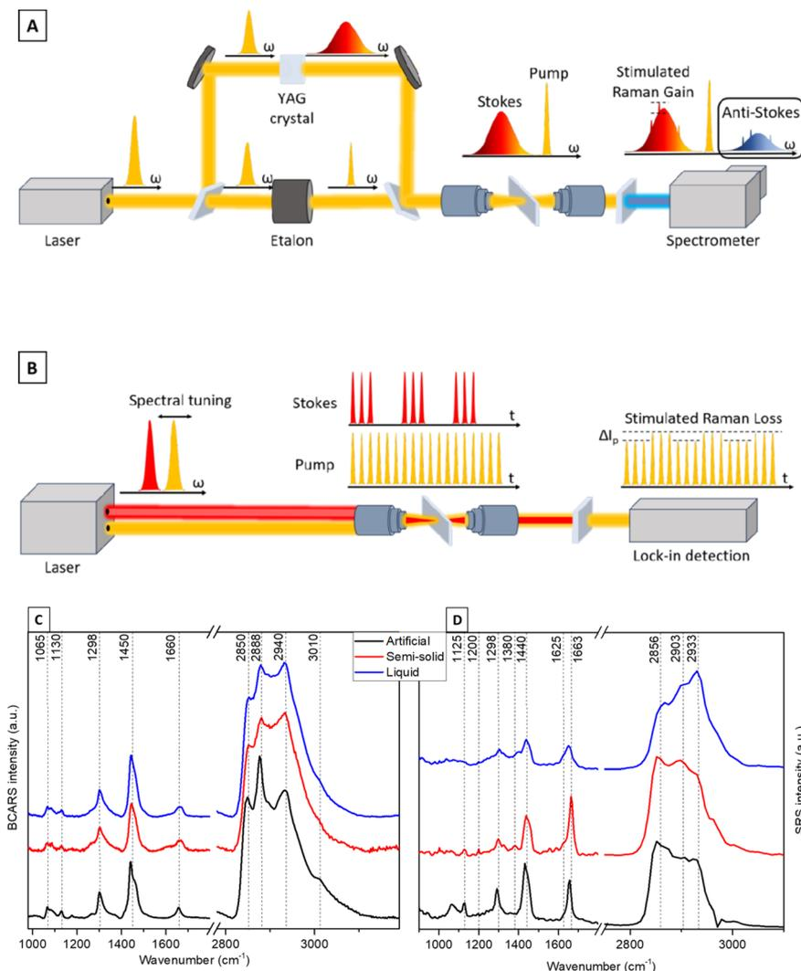
**Fig. 4** Schematic illustrations of (A) the home-built BCARS and (B) SRS setups. Averaged (C) BCARS and (D) SRS spectra of artificial (black), semi-solid (red) and liquid (blue) cerumen. Wavenumber range between 900 and 3200  $\text{cm}^{-1}$ . The spectra are cut in the silent region between 1800 and 2750  $\text{cm}^{-1}$ . Spectra are offset for clarity.
