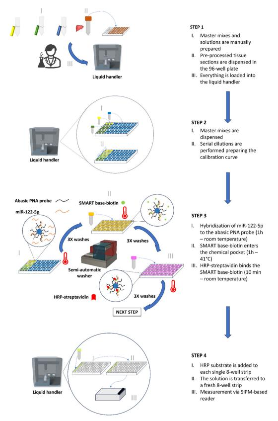
Fig. 1 SA-ODG platform workflow. STEP 1: equipping the liquid handler with master mixes, solutions and the homogenised tissue sections into the 8-well strips in a support frame with 96 spaces; STEP 2: calibration curve and sample testing preparation; STEP 3: DCL reaction for SMART basebiotin incorporation and HRP-streptavidin labelling; STEP 4: chemiluminescent signal measurement via the SiPM-based reader.
