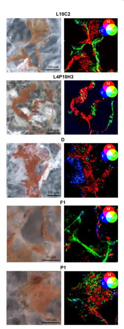
Fig. 5 The OM images and the RGB false colour  $\mu$ -XRPD combination maps of one area of each of the analysed samples are shown. The phase distribution of minium (M), hydrocerussite (HC), cerussite (C) and plattnerite (P) are highlighted.
