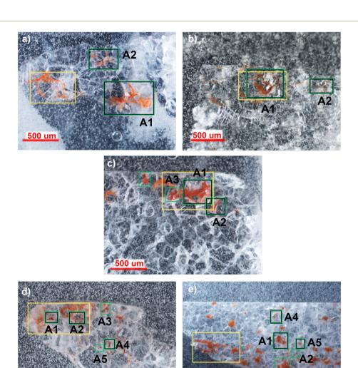
Fig. 2 Optical microscope images (4-10x magnification) of the thin sections coming from the Duomo and the Baptistery of Florence (D, L10-C2, L4P10H3) (a, b, c) and from monumental fountains in Villa La Petraia (P1, F1) (d, e). Green squares in all the images, refer to μ-XRPD and μ-XRF measurements while black squares refer to μ-Raman analysed areas. In yellow squares SEM-EDS and FTIR chemical imaging analysed areas.
