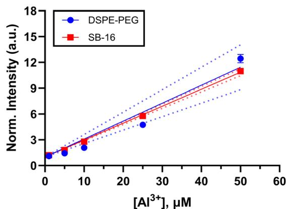
Fig. 2 Response of the Al<sup>3+</sup> sensors made with DSPE-PEG and SB-16 to analyte ranging from 1 μM to 50 μM. While there is a small variation, both responses show a similar trend (two-tailed *t*-test, 95% C.I.,  $p = 0.1134 > 0.05$ ). Note, the data was normalized to the response at 1 μM, also where not visible the errors bars are smaller than the data points ( $n = 3$ ).
