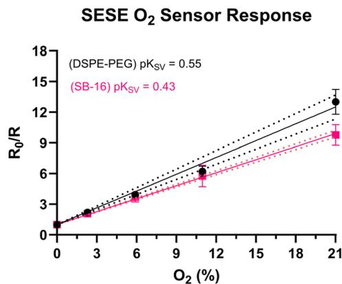
**Fig. 3** The pseudo-Stern–Volmer calibration curve shows that SESE O<sub>2</sub> sensors fabricated with DSPE-PEG are more sensitive to oxygen changes than its SB-16 counterpart as evidenced by the higher  $pK_{SV}$  value (statistical difference verified *via* two-tailed *t*-test, 95% C.I.,  $p = 0.0435 < 0.05$ ). Where not visible the error bars are smaller than that of the data points ( $n = 3$ ).
