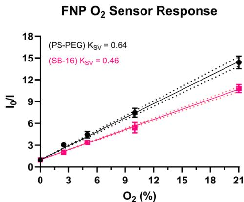
**Fig. 4** Stern–Volmer response from the O<sub>2</sub> sensors fabricated using FNP at varying O<sub>2</sub> concentrations. The sensors made with PS-PEG show a more sensitive response to changes in oxygen than its SB-16 counterpart (statistical difference verified *via* two-tailed *t*-test, 95% C.I.,  $p = 0.0037 < 0.05$ ). Both sensors were excited at 405 nm and the emissions observed 650 nm. Where not visible the error bars are smaller than those of the data points ( $n = 3$ ).
