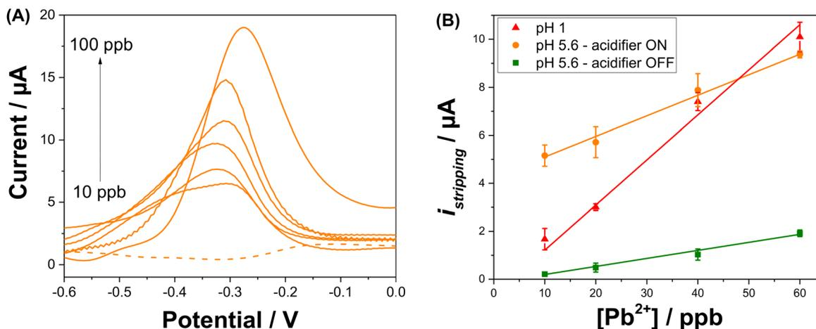
**Fig. 5** (A) SWV of different  $\text{Pb}^{2+}$  concentrations (10, 20, 40, 60, 80, 100 ppb) recorded in 0.1 M  $\text{NaNO}_3$  (pH 5.6) with *in situ* acidification, according to the optimized procedure. (B) Calibration curves for anodic stripping peak current vs.  $\text{Pb}^{2+}$  concentration at pH 1 ( $\blacktriangle$ ), and at pH 5.6 when the acidifier is ON ( $\bullet$ ) and OFF ( $\blacksquare$ ).
