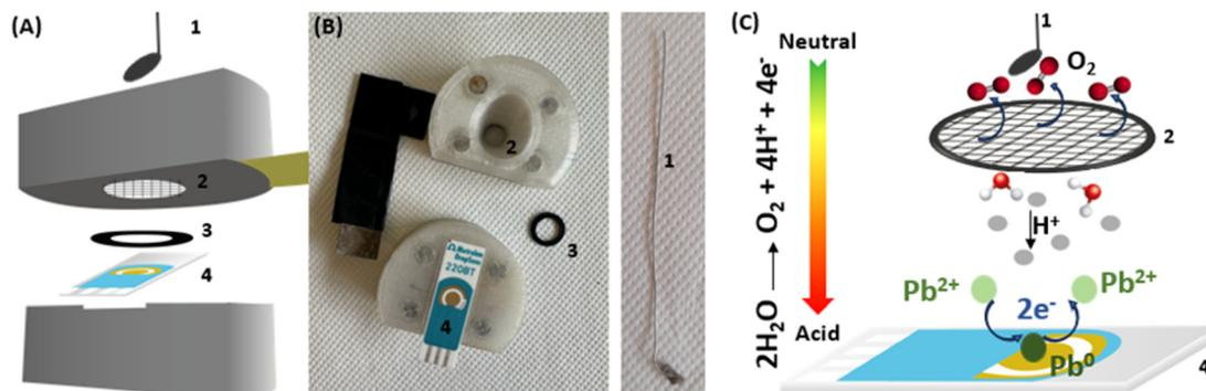
**Fig. 1** (A) Schematic representation, (B) photograph, and (C) operating principle of the 3D printed electrochemical cell with integrated pieces: (1) external auxiliary Pt electrode, (2) acidifier (Pt grid), (3) spacer, (4) screen printed electrode 220BT (gold sensing electrode and silver reference electrode).
