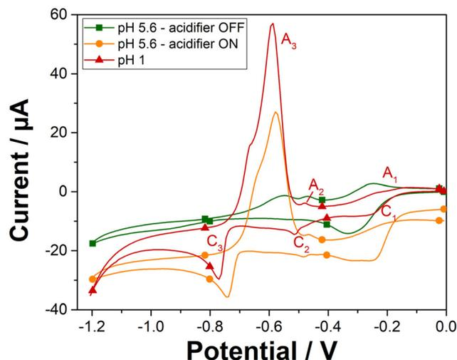
Fig. 3 Cyclic voltammograms of gold electrode obtained in 100 ppm  $\text{Pb}^{2+}$  at pH 1 (red triangle curve), and at pH 5.6 with the acidifier switched off (green square curve), and with the acidifier switched on (orange circle curve). Scan rate  $50 \text{ mV s}^{-1}$ .
