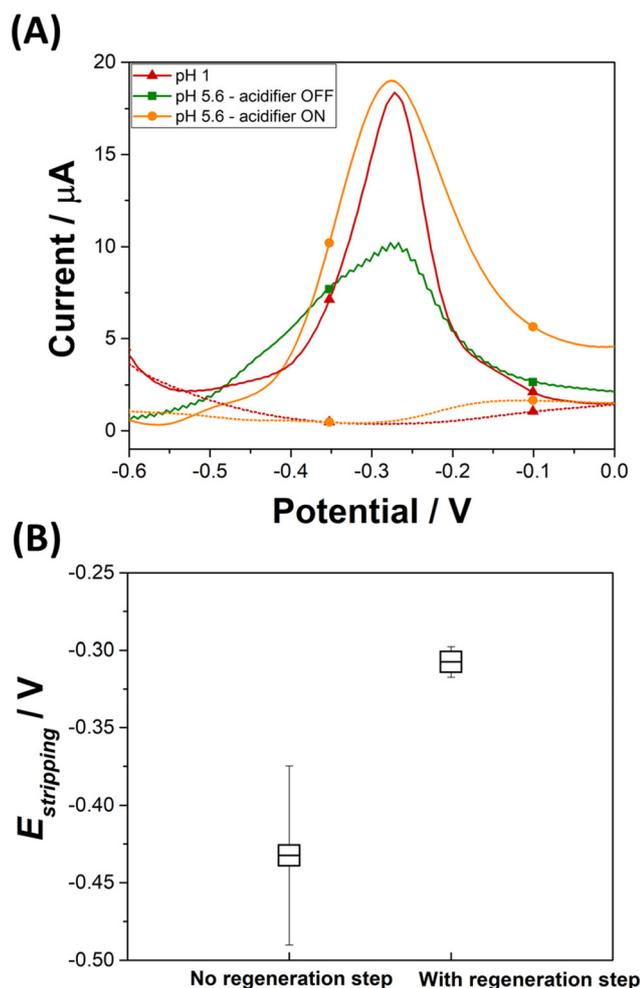
**Fig. 4** (A) SWV of 100 ppb  $\text{Pb}^{2+}$  on a gold electrode in  $\text{HNO}_3$  (pH 1) (red triangle curve) and in 0.1 M  $\text{NaNO}_3$  (pH 5.6) with the acidifier switch off (green square curve) and on (orange circle curve). (B) Average of stripping peak potentials values obtained with ( $N = 20$ ) and without ( $N = 80$ ) regeneration step of the acidifier.
