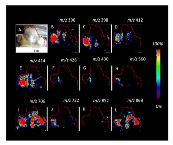
Fig. 12 Imaging DESI-MS of an infected potato sprout imprinted on tape, 8 d after inoculation. Localization of the new metabolites (A-L) biosynthesized after fungus invasion can be observed. The infected potato sprout is imprinted directly on tape without further manipulation. The red outline indicates the portion of the sprout and the tuber imaged. Figure adapted and reprinted with permission from ref. 101 with permission from American Chemical Society, copyright (2015).
