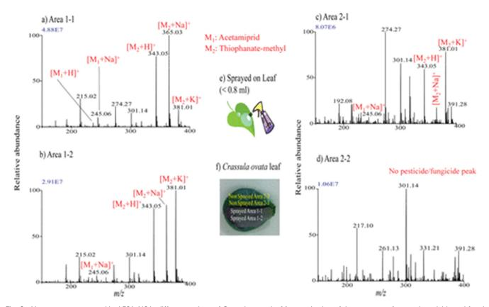
Fig. 6 Mass spectra measured by LESA-MS in different regions of *Crassula ovata* leaf for monitoring of the presence of sprayed pesticide and fungicide after a week. (a–d) Mass spectra measured at the different regions: area 1-1 (a), area 1-2 (b), area 2-1(c), and area 2-2 (d), shown in panel (f). (e) Schematic for the spraying procedures of pesticide and fungicide mixture solution on leaf. Reprinted with permission from ref. 72 with permission from American Chemical Society, copyright (2013).
