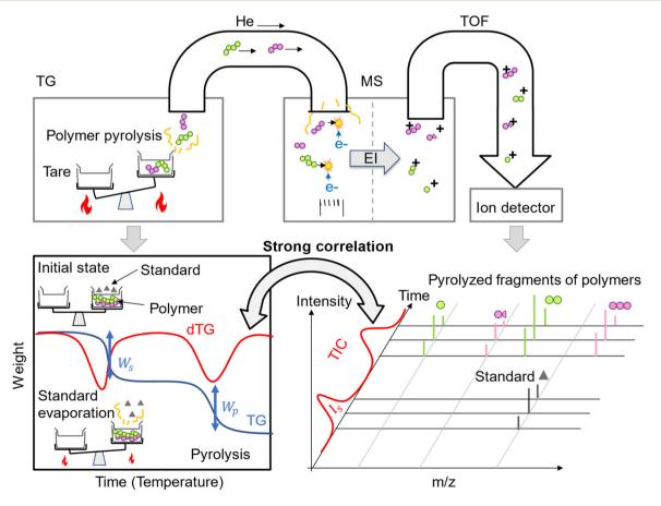
Fig. 1 TG-TOFMS setup for TG-RQMS. The weight and MS spectra are recorded every second. The synchronous analysis of instantaneous weight loss (dTG) and MS spectra allow the estimation of ionization efficiencies of pyrolyzed fragments for improving the RQMS accuracy.
