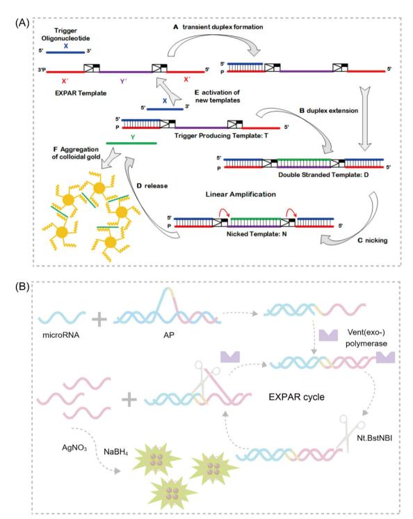
Fig. 7 Schematic representation of MNC-based approaches. (A) A novel design combining EXPAR and gold-nanoparticle visualization for the detection of miRNAs. (B) Fluorometric determination of miRNAs using arched probe-mediated EXPAR combined with DNA-templated silver nanoclusters. (106)
