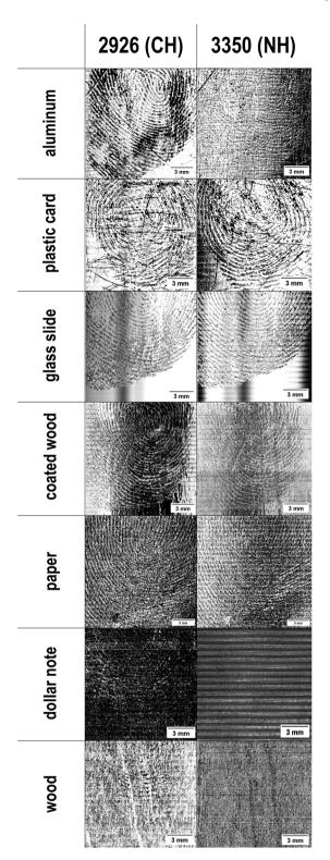
**Fig. 6** Images acquired based on the CH and NH absorbance bands of latent fingerprints scanned on aluminum, a plastic card, a glass slide, wood (coated and uncoated), a dollar note and paper using the MIR system.
