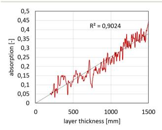
Fig. 10 Linear absorbance correlation to different layer thicknesses of adeps lanae scanned with the MIR system.
