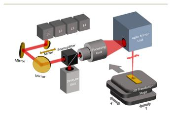
Fig. 1 Schematic of the MIR scanning system with inbuilt lasers of wavenumbers 3700 cm<sup>-1</sup> (L1), 3350 cm<sup>-1</sup> (L2), 2926 cm<sup>-1</sup> (L3) and 2790 cm<sup>-1</sup> (L4).
