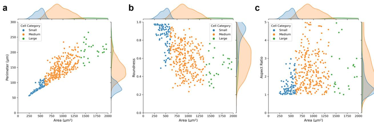
**Fig. 3** Scatter plots of typical cell morphological features, cell perimeter (a), roundness (b), and aspect ratio (c) versus cell area, with a total cell count ( $N = 398$ ) indicated. The blue, orange, and green dots in the scatter plots represent small, medium, and large cells, respectively. Corresponding density distribution plots for each morphological feature are shown on the top and right panels.
