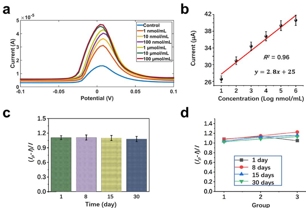
Fig. 4 General performance of the CA NF-decorated PBSP sensor in detecting glucose. (a) DPV curves and (b) the calibration curve; (c) stability evaluation of the sensor; (d) repeatability test of the sensor ( $n = 3$ ).
