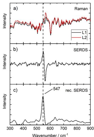
Fig. 9 Illustration of serds employed as physical approach and mathematical procedure used to reconstruct the final serds spectrum of S3.
