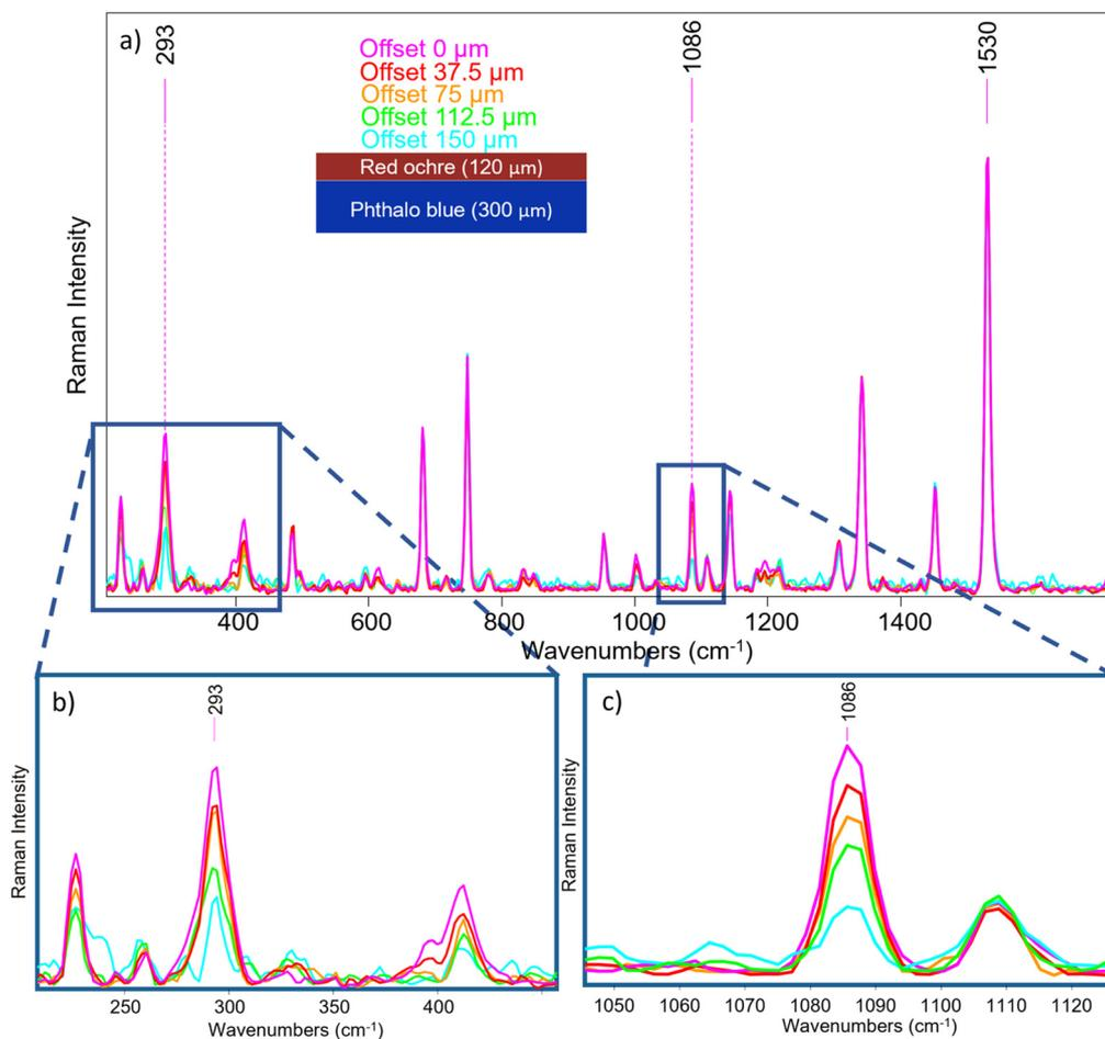
**Fig. 8** (a) Micro-SORS measurement of S2 where all spectra have been normalized to the 1530  $\text{cm}^{-1}$  band of the bottom layer. The SORS effect is clearly visible for raman bands of (b) red ochre and (c) calcite.
