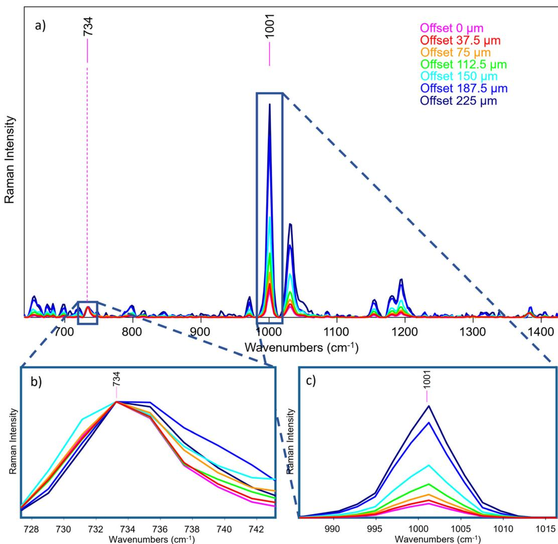
**Fig. 6** (a) Portable fibre bundle micro-SORS measurement of S1; (b) all spectra have been normalized to the Teflon band (top layer) at 734  $\text{cm}^{-1}$ ; (c) relative intensity increase of the polystyrene signal (bottom layer) (i.e. at 1001  $\text{cm}^{-1}$ ) as the offset increases.
