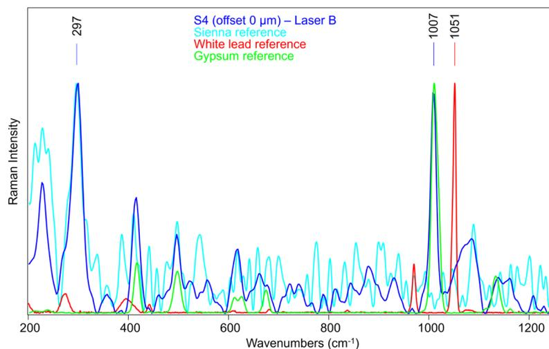
**Fig. 11** Offset 0 spectrum of S4 analysed with the system coupled with Laser B, compared with the reference spectra of the Sienna pigment (top layer), white lead (bottom layer) and gypsum (preparation layer). The main band of Sienna pigment is clearly visible ( $297\text{ cm}^{-1}$ ), along with the gypsum band at  $1007\text{ cm}^{-1}$ . No white lead signal can be seen.
