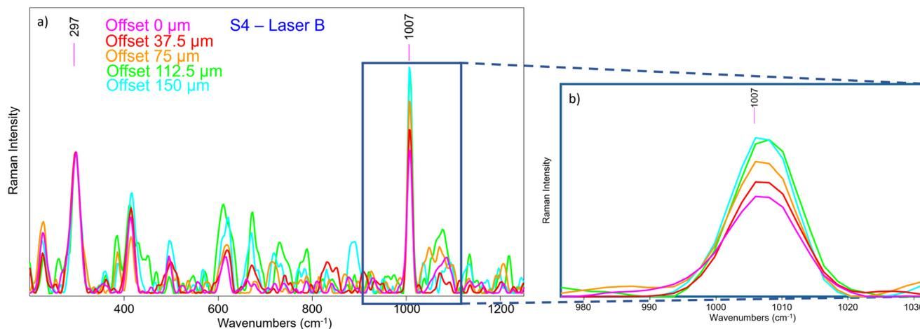
**Fig. 12** (a) micro-SORS series acquired with the system coupled with Laser B in S4. All spectra have been normalized to the Sienna pigment characteristic band at  $297\text{ cm}^{-1}$ ; (b) micro-SORS effect is visible through the increase of the gypsum ( $1007\text{ cm}^{-1}$ ) band of the preparation layer at the increasing of the offset.
