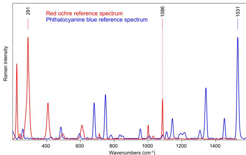
**Fig. 7** Reference spectra of the two painted layers of S2, directly acquired on parts of the sample where they are not overlapped. The reference frequencies for each compound are indicated: 291  $\text{cm}^{-1}$  for red ochre, 1086  $\text{cm}^{-1}$  for calcite and 1531  $\text{cm}^{-1}$  for phthalocyanine blue.
