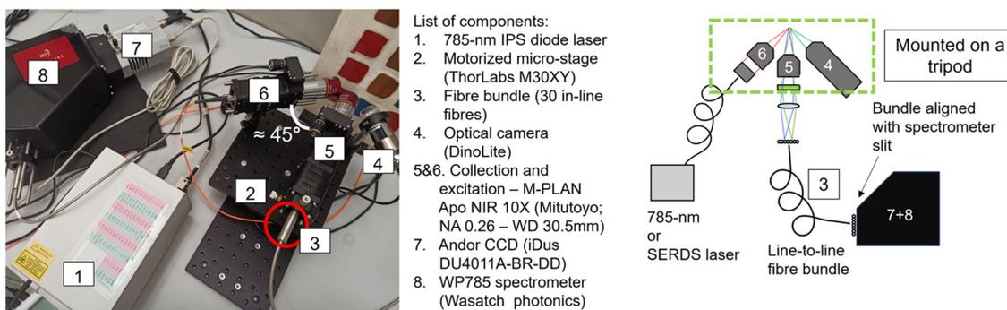
Fig. 2 Photo (a) and schematics (b) of the prototype with each component labelled.
