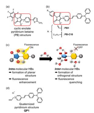
Fig. 1 (a) The pyridinium betaine (PB) structure, as reported by Suzuki and Yagi et al.49 (b) The molecular design employed in the present study. (c) Concept underlying the fluorescence-based water detection (HB: Hydrogen Bond). (d) The quaternary pyridinium structure QP1, which was used as a reference compound.
