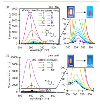
Fig. 3 Fluorescence spectra of the dye-immobilised membranes (a) **PB1**-mem ( $\lambda_{ex}$  = 490 nm,  $\lambda_{fl}$  = 630 nm) and (b) **QP1**-mem ( $\lambda_{ex}$  = 460 nm,  $\lambda_{\rm fl}$  = 630 nm) in THF/water solvents.
