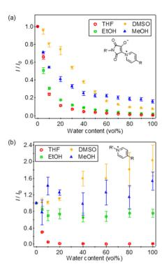
Fig. 4 Relative fluorescence intensities of the dye-immobilised membranes (a) PB1-mem ( $\lambda_{\rm ex}=490$  nm,  $\lambda_{\rm fl}=630$  nm) and (b) QP1-mem ( $\lambda_{\rm ex}=460$  nm,  $\lambda_{\rm fl}=630$  nm) in water mixed with THF, DMSO, ethanol (EtOH), and methanol (MeOH).
