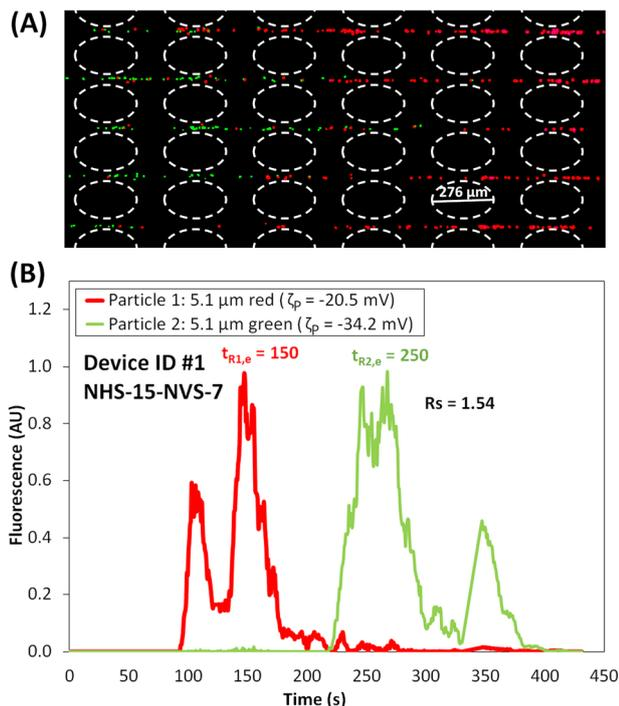
**Fig. 2** (A) Image of the microparticles in the post array of the iEK device, where the particles are forming “zones” as the red particles are migrating faster and ahead of the green particles (see ESI Video S1†). (B) Electropherogram of the microparticle separation obtained with NHS = 15 and NVS = 7. The applied potential was  $V_p = 800$  V, at 1.1 Hz and a DC bias of 300 V.
