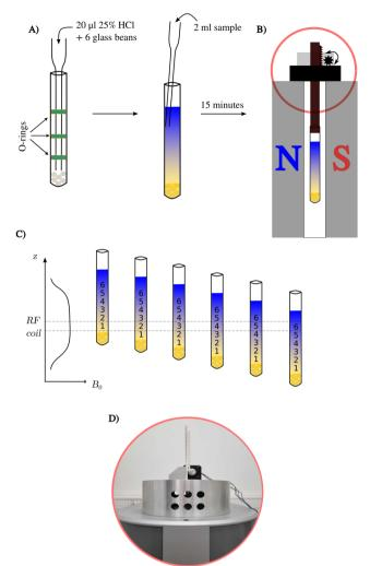
Fig. 1 Scheme of a pH gradient experiment using 43 MHz BT-NMR. (A) General sample preparation procedure, (B) sample in the SWAPE device inside a BT-NMR spectrometer, (C) idea of measuring a series of <sup>1</sup>H NMR spectra, and (D) a photo of the SWAPE motor marked in red on panel (B).
