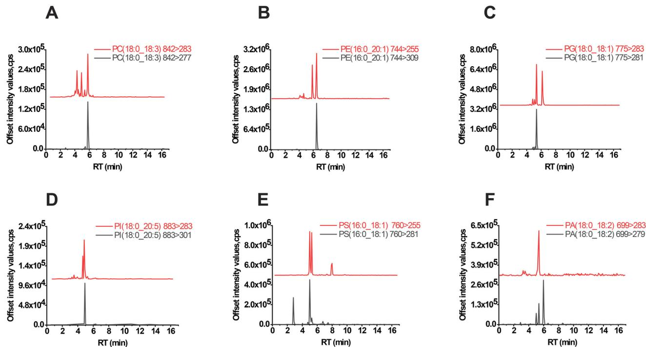
**Fig. 3** MRM validation for phospholipids. TIC of the representative subclass of phospholipids such as PC(18:0\_18:3) (A), PE(16:0\_20:1) (B), PG(18:0\_18:1) (C), PI(18:0\_20:5) (D), PS(16:0\_18:1) (E) and PA(18:0\_18:2) (F). *x* represents the RT value (min), and *y* represents the offset intensity values (cps).
