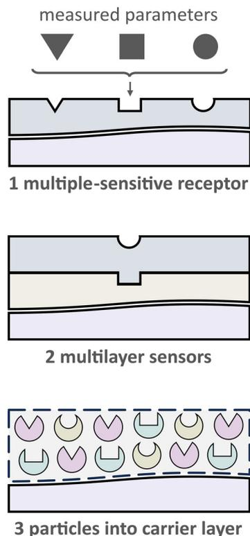
**Fig. 5** Schematic of the three most common designs for creating multiparameter optical sensors *via* different recognition options: (1) multiple-sensitive receptor, (2) multilayer sensors, (3) (nano)particles into carrier layer.
