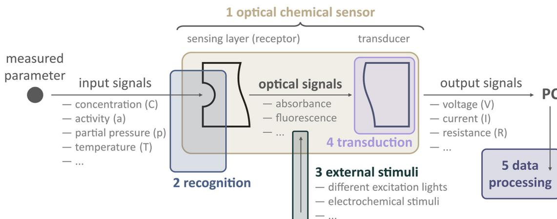
**Fig. 3** Schematic depiction of measurements conducted using optical chemical sensors. The color blocks and numerical annotations indicate the specific sites enabling the simultaneous analysis of multiple parameters, presented in the order listed (see text for more details). PC denotes the personal computer.
