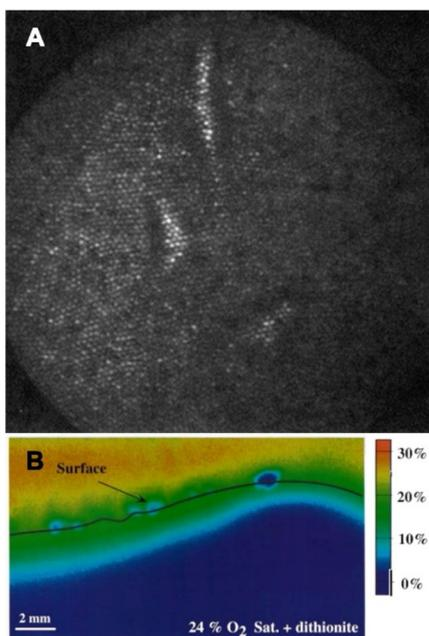
**Fig. 2** Different designs of multiparameter optodes. (A) Fiber-bundle sensor design: polyHema/fluorescein-modified imaging fiber with mouse fibroblast cells.<sup>42</sup> (B) Planar 2D sensor design ("Glud's design"): calibrated images of the O<sub>2</sub> distribution at the sediment-water interface with sodium dithionite grains added.<sup>22</sup> Reprinted with permission from ref. 42. Copyright 1995 American Chemical Society.
