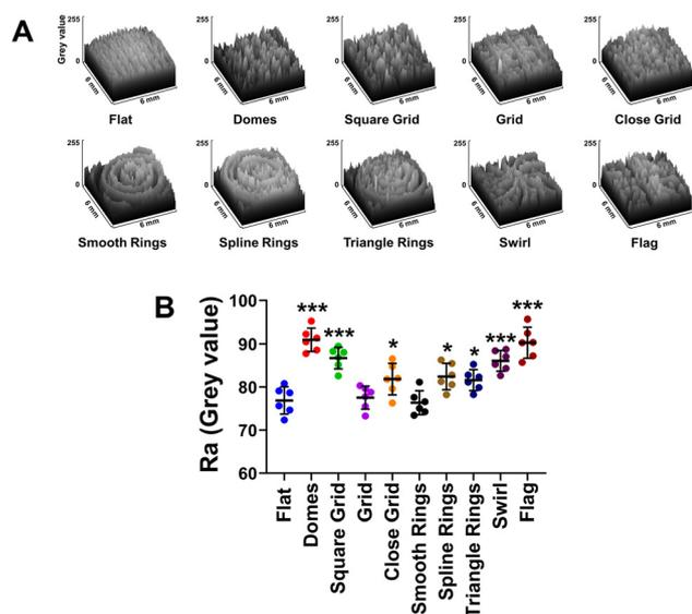
**Fig. 5** Surface roughness analysis. (A) The surface profile of a print layer of each pattern. (B) Analysis of the average surface roughness ( $A_b$ ) measured in grey values obtained from three print layers of the electrodes. Data shown as mean  $\pm$  SD, where  $n = 6$ , \* $p < 0.05$  and \*\*\* $p < 0.001$ .
