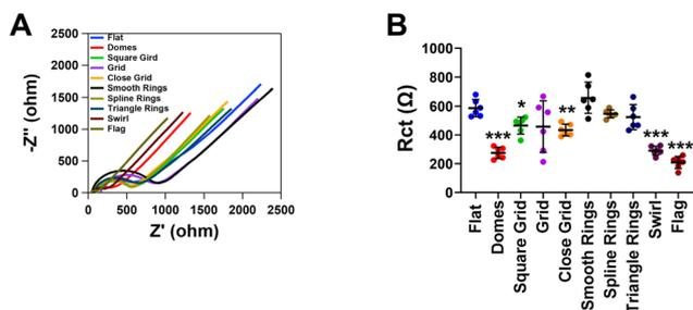
**Fig. 3** Electrochemical impedance spectroscopy measurements. (A) Nyquist plots for the electrodes with various patterned surfaces in which the (B) charge-transfer resistance ( $R_{ct}$ ) was determined. Data are presented as mean  $\pm$  SD, where  $n = 6$ , \* $p < 0.05$ , \*\* $p < 0.01$  and \*\*\* $p < 0.001$ .
