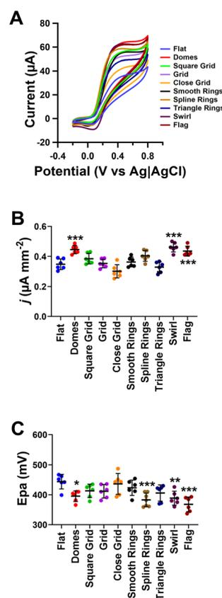
**Fig. 4** Responses of 3D printed CB/PLA electrodes with various patterned surfaces in 1 mM Dopamine. (A) Cyclic voltammograms of 1 mM dopamine in 0.1 M PBS at  $0.05 \text{ V s}^{-1}$ . (B) Current density and (C) anodic peak potential ( $E_{pA}$ ). Data shown as mean  $\pm$  SD, where  $n = 6$ , \* $p < 0.05$ , \*\* $p < 0.01$  and \*\*\* $p < 0.001$ .
