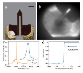
Fig. 3 AFM tuning fork and cantilever. Visible light image (a) with 100 µm scale bar. X-ray TX projection (b) showing the tip in front of the zone plate optics and the central stop. Normalized resonance sweep in air (blue) and under vacuum (orange) (c), showing the expected increase of the Q factor under vacuum. Tip sample approach curve (d) showing a sudden decrease of the phase at the tip-sample mechanical contact point, indicating a rapid shift of the resonance.
