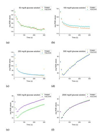
**Fig. 6** Correlation between time and measured average RGB values and the comparison between ImageJ and glucose detector measurements. (a) 50 mg dL $^{-1}$  glucose concentration. (b) 100 mg dL $^{-1}$  glucose concentration. (d) 500 mg dL $^{-1}$  glucose concentration. (e) 1000 mg dL $^{-1}$  glucose concentration. (f) 2000 mg dL $^{-1}$  glucose concentration.
