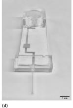
Fig. 2 Actual pictures of a microfluidic channel and molds for the PDMS components. (a) Microfluidic channel. (b) PDMS micropumps and 3D-printed molds. (c) PDMS extension part, capillary and 3D-printed molds. (d) Microfluidic device after assembly of all components.
