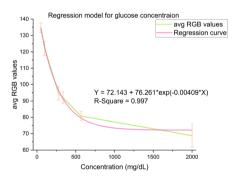
Fig. 7 Regression curve based on glucose detector measurements.
