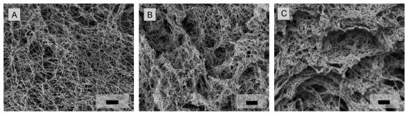
Fig. 7 SEM micrographs of collagen, alginate and IPN hydrogels. (A) Fibrillar collagen type 1 at a concentration of 2 mg ml<sup>-1</sup>. (B) Alginate hydrogel with 20 mM of the Ca<sup>2+</sup> crosslinker. (C) IPN hydrogel with 20 mM of the Ca<sup>2+</sup> crosslinker. The scale bars denote 20 µm.
