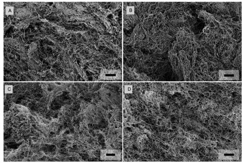
Fig. 8 SEM micrographs about the topology of softer and stiffer IPN hydrogels. (A) and (B) Softer IPN hydrogels with 7.5 mM of the Ca<sup>2+</sup> crosslinker. (C) and (D) Stiffer IPN hydrogels with 20 mM of the  $Ca^{2+}$  crosslinker. The scale bars denote 10  $\mu m$ .
