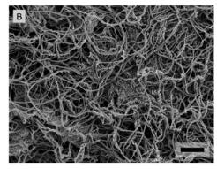
Fig. 9 High-resolution SEM micrographs of homogeneously distributed collagen type 1 mesh within the porous network of softer and stiffer IPN hydrogels. (A) Softer IPN hydrogels with 7.5 mM of the  $Ca^{2+}$  crosslinker. (B) Stiffer IPN hydrogels with 20 mM of the  $Ca^{2+}$  crosslinker. The scale bars denote 2  $\mu$ m.
