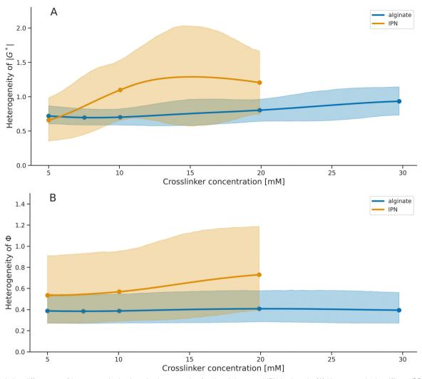
Fig. 10 Relative differences of heterogeneity in viscoelastic properties for the alginate and IPN hydrogels. (A) Heterogeneity in stiffness ( $|G^*|$ ) and (B) heterogeneity in phase angle  $(\Phi)$  with respect to crosslinker concentration. The shaded area is the 95% credible interval, and the darker lines are the calculated means. Scatter points depict the crosslinker concentrations at which the hydrogels were measured, while the regions in between are the modelled estimates
