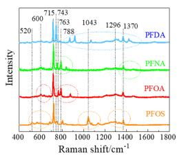
Fig. 2 The Raman spectra of selected PFAS powders.
