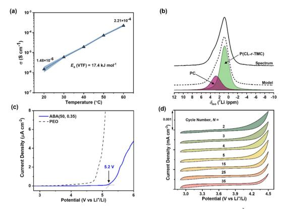
Fig. 3 (a) Temperature-dependence of ionic conductivity for ABA (50, 0.35)/17 wt% LiTFSI. (b) Solid-state <sup>7</sup>Li NMR spectrum with peak deconvolution to PC and P(CL-r-TMC) phases. (c) Oxidative stability vs. Li metal and stainless-steel counter electrode measured by LSV at 60 °C, 0.1 mV s<sup>-1</sup> scan rate. (d) CV at 0.5 mV s<sup>-1</sup> scan rate recorded over 35 cycles.
