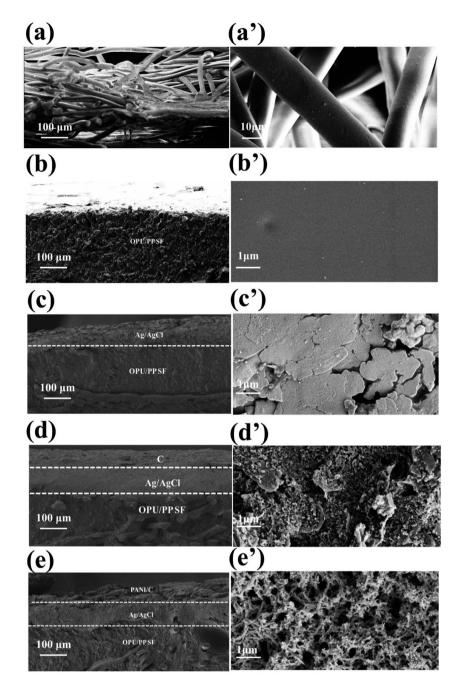
Fig. 3 SEM images of the (a-e) cross-section and (a'-e') surface of PP SF, OPU/PP SF, Ag/AgCl@OPU/PP SF, C@OPU/PP SF, and 3D PANI pH sensors.
