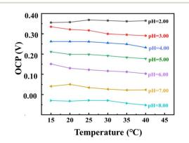
Fig. 8 OCP-temperature curves of 3D PANI pH sensors in buffer solutions with the pH changing from 2.00 to 8.00 in the normal state.
