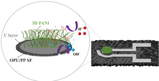
Fig. 11 Scheme of the protonation-deprotonation (a) mechanism and (b) pathway for 3D PANI.
