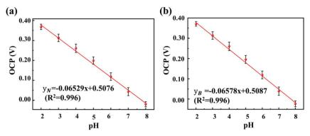
Fig. 9 Fitted OCP-pH curves of 3D PANI sensors in the (a) normal state and (b) bent state in pH 2.00-8.00 buffer solutions during the reproducibility test.
