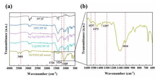
Fig. 4 (a) FT-IR spectra of PP SF, OPU/PP SF, Ag/AgCl@OPU/PP SF, C@OPU/PP SF and 3D PANI pH sensors, and (b) magnified FT-IR spectrum with the wavenumber ranging from  $1600 \text{ to } 600 \text{ cm}^{-1}$ .
