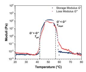
Fig. 5 A representative moduli–temperature plot of BCACB pentablock terpolymer at 10 wt% in PBS, tested under an angular frequency of 1.0 rad s $^{-1}$ , a strain of 1.0%, and a heating rate of 1.0 °C min $^{-1}$ .
