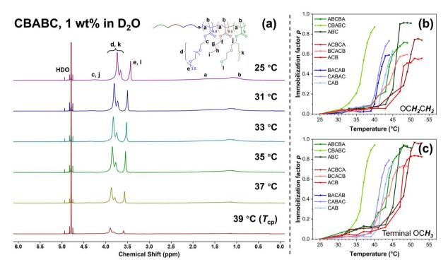
Fig. 3 (a) The VT- $^{1}$ H NMR spectra of CBABC polymer at 1 wt% in D<sub>2</sub>O solution at representative temperatures from 25 °C to 39 °C, and the temperature–dependent immobilisation factor p of the protons from (b) the OCH<sub>2</sub>CH<sub>2</sub> and (c) the terminal OCH<sub>3</sub> in the side chain of the poly(DEGMA300) and poly(DEGMA) blocks in 1 wt% polymer solution in D<sub>2</sub>O.
