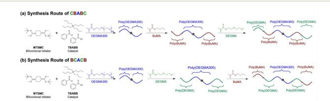
Scheme 2 Representative synthesis routes of CBABC and BCACB pentablock terpolymers via one-pot GTP, where A, B, and C blocks consist of OEGMA300, BuMA, and DEGMA, respectively.
