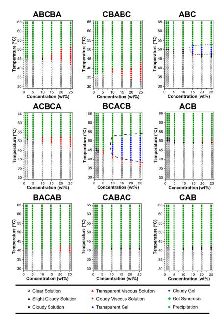
Fig. 4 Phase diagrams of the polymer in PBS (pH = 7.4, 1x) at 1, 2, 5, 10, 15, 20, and 25 wt%. The heating rate was approximately 1 °C min<sup>-1</sup>.
