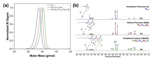
Fig. 1 (a) GPC traces in THF–Et<sub>3</sub>N mixture (95–5 vol%) and (b) <sup>1</sup>H NMR spectra in CDCl<sub>3</sub> of the CBABC pentablock terpolymers and its precursors. "O", "B", and "D" are the abbreviations of OEGMA300 (block A), BuMA (block B), and DEGMA (block C), respectively.
