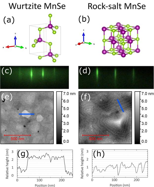
**Fig. 1** Comparison of the structural characteristics of the top surface of wurtzite MnSe (left column, sample WZ3) and rock-salt MnSe (right column, sample RS1). Atomic structure diagrams of (a) wurtzite and (b) rock-salt MnSe. (c) and (d) RHEED images taken just at the end of the growth. (e) and (f) AFM topography scans and (g) and (h) profiles of the relative height along the blue lines indicated in the AFM images.
