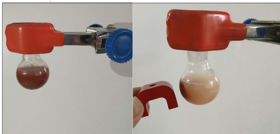
Fig. 7 Recyclability of \text{Fe}_3\text{O}_4@\text{SiO}_2@\text{SBA-3}@_2\text{-ATP-Cu} .
