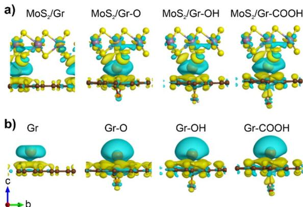
Fig. 2 Charge density difference plot between Na and neighboring (a) heterogeneous bilayers and (b) monolayers (isosurface level:  $0.0008 \text{ eV } \text{\AA}^{-3}$ ). The blue and yellow surface densities represent charge depletion and accumulation, respectively.
