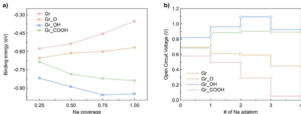
Fig. 5 (a) Average binding energies of the Na intercalation in graphene and rGO bilayer plotted with respect to Na coverage. (b) The voltage profile MoS<sub>2</sub>/Gr and MoS<sub>2</sub>/rGO as a function of Na adatom number.
