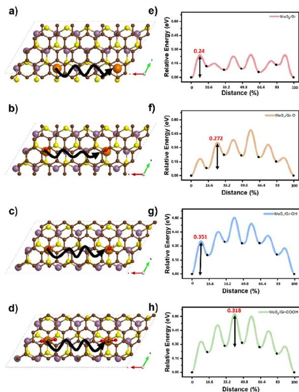
Fig. 4 (a–d) Na atom diffusion pathways (solid line) and (e–h) energy profiles for Na diffusion in MoS<sub>2</sub>/Gr, MoS<sub>2</sub>/Gr-O, MoS<sub>2</sub>/Gr-OH, and MoS<sub>2</sub>/Gr-COOH.
